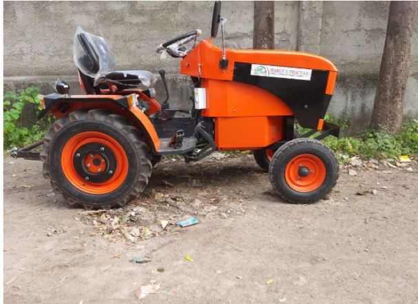
Side profile of the 18 hp e-tractor
